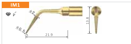
IM1 Diamond Bone Perforation. Conical surgery tip with diamond layer for bone perforation. Recommended for pilot osteotomy in extraction sites and to check the alignment of the axis of PIN IM1 preparations.
